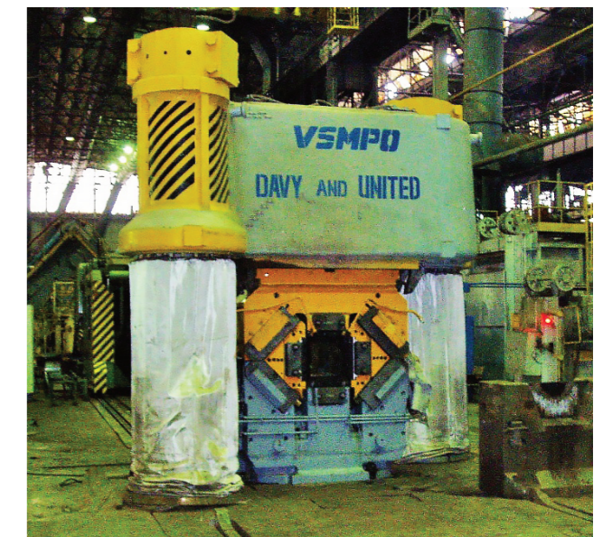
FDFD employed on a 25MN press to forge titanium billets at VSMPO-AVISMA plant
