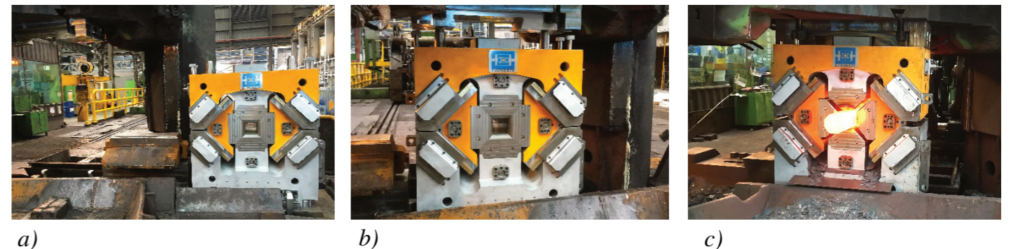
Quick change of the four-die forging device on a 22 MN press (Korea)
