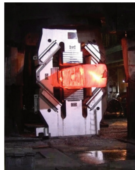
Forging a square section forging in FDFD on a 30 MN press (Japan)
